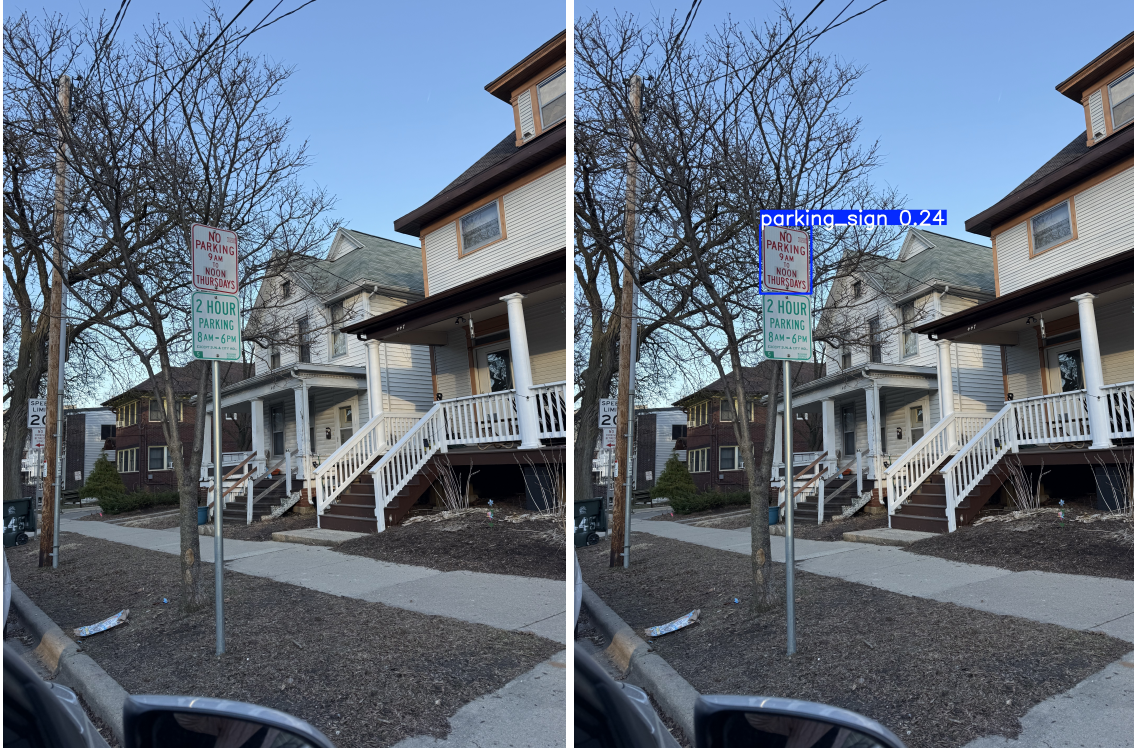
Figure 15: Effect of input resolution on detection. Left: Higher resolution (imgsz=1280) input where the parking sign is missed. Right: Lower resolution (imgsz=160) input where the same sign is detected.
