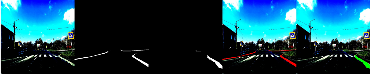
Figure 18: Example qualitative curb segmentation result. The model captures the curb location, but the prediction remains thin and fragmented rather than forming a dense continuous region.
