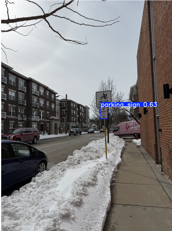
Figure 13: Qualitative examples from manually collected images. These illustrate successful detections and also the tendency to localize the most visually salient sub-sign rather than the full sign assembly (for example, the image on the right where only the P sign is detected).
