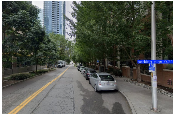
Figure 13: Qualitative examples from manually collected images. These illustrate successful detections and also the tendency to localize the most visually salient sub-sign rather than the full sign assembly (for example, the image on the right where only the P sign is detected).
