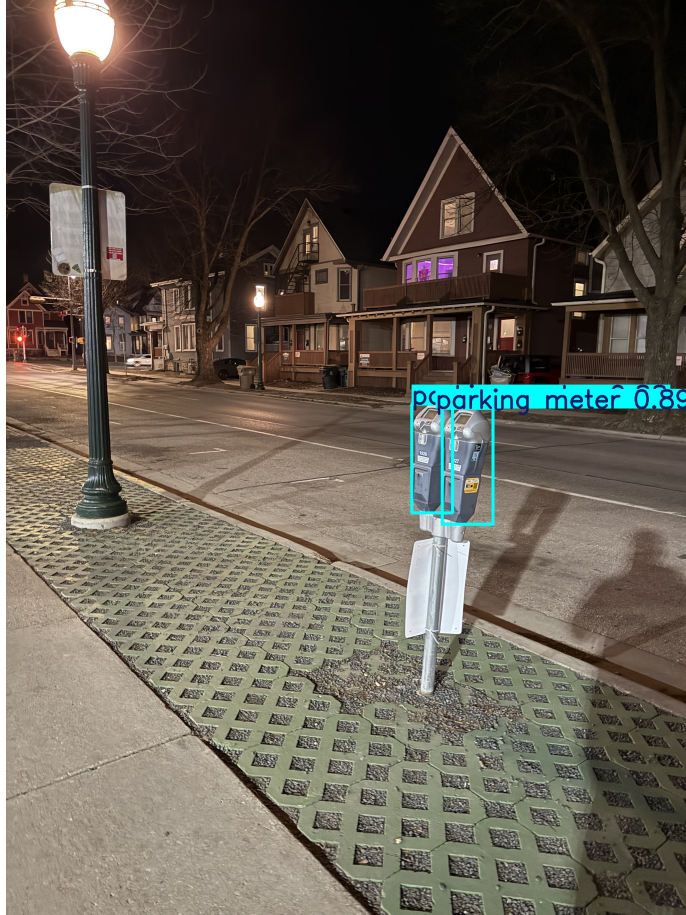
Figure 10: Example qualitative parking-meter detection from a manually collected image. The COCO-pretrained YOLO11x model successfully detects the parking meter in a close-view nighttime scene.
