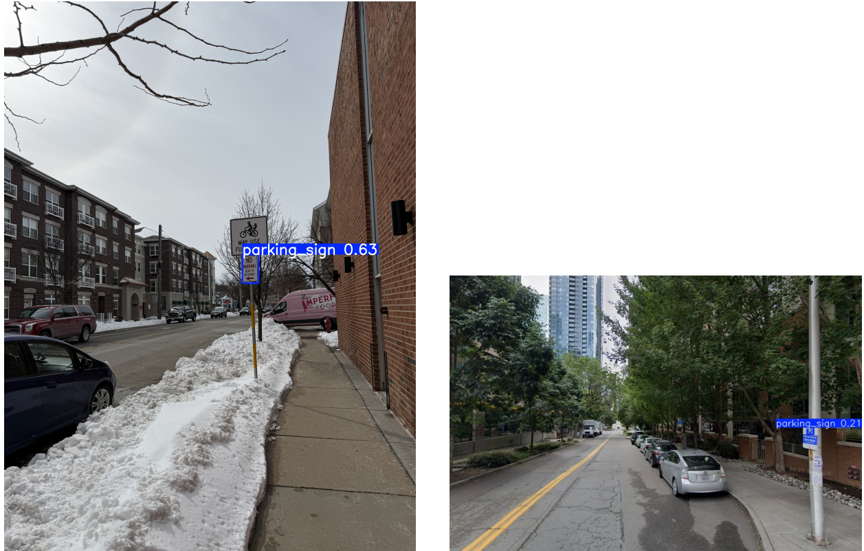
Figure 6: Qualitative examples from manually collected images. These illustrate successful detections and also the tendency to localize the most visually salient sub-sign rather than the full sign assembly (like image on right which only detects the 'P').
